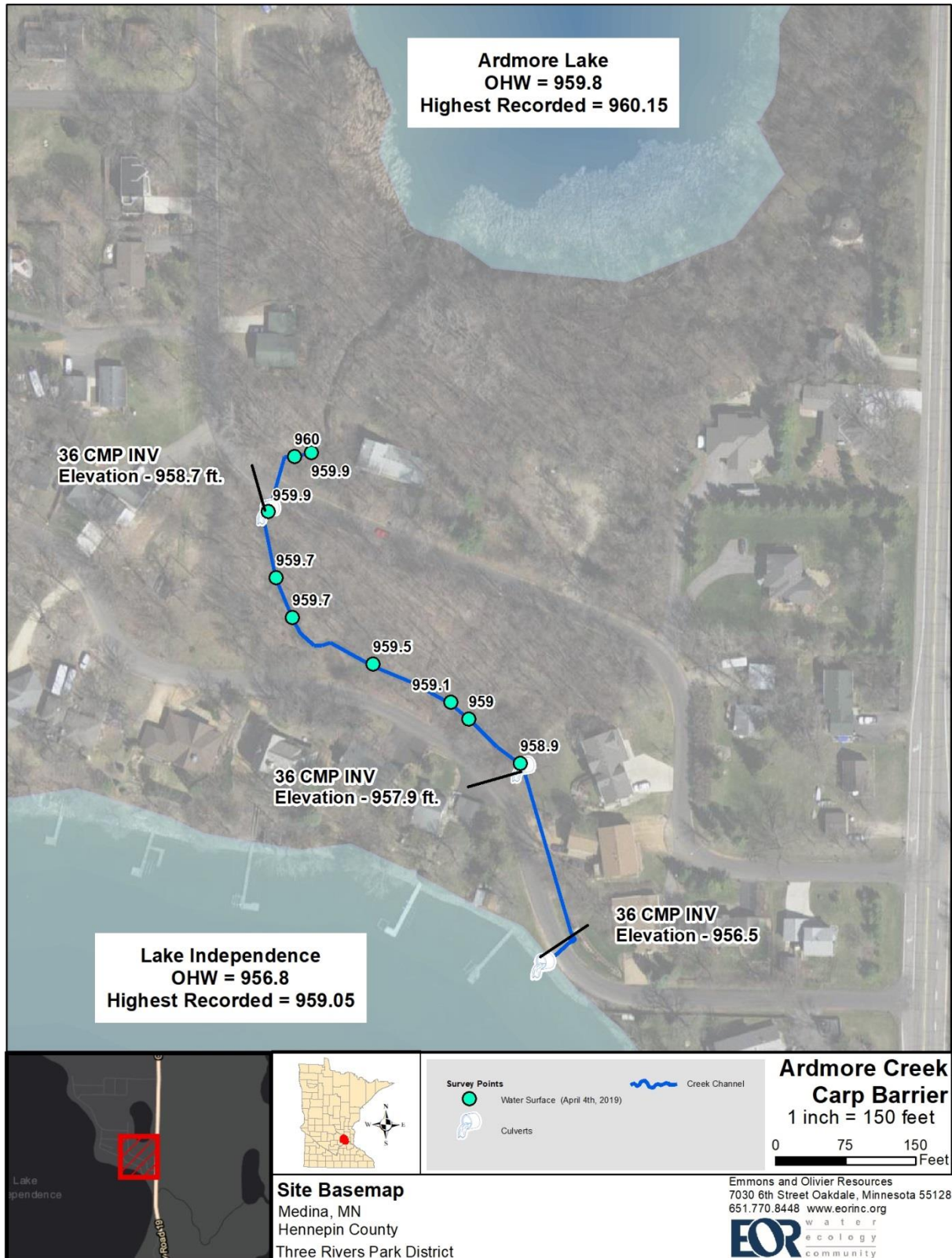
Figure 1. Ardmore Channel Profile and Culvert Elevations (Point Elevations Represent Water Surface Elevations)
